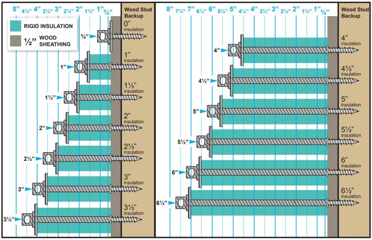
**THERMAL Concrete Seal Tie™** is an innovative single screw veneer tie suitable for use with concrete, CMU, wood stud, or brick backup.
