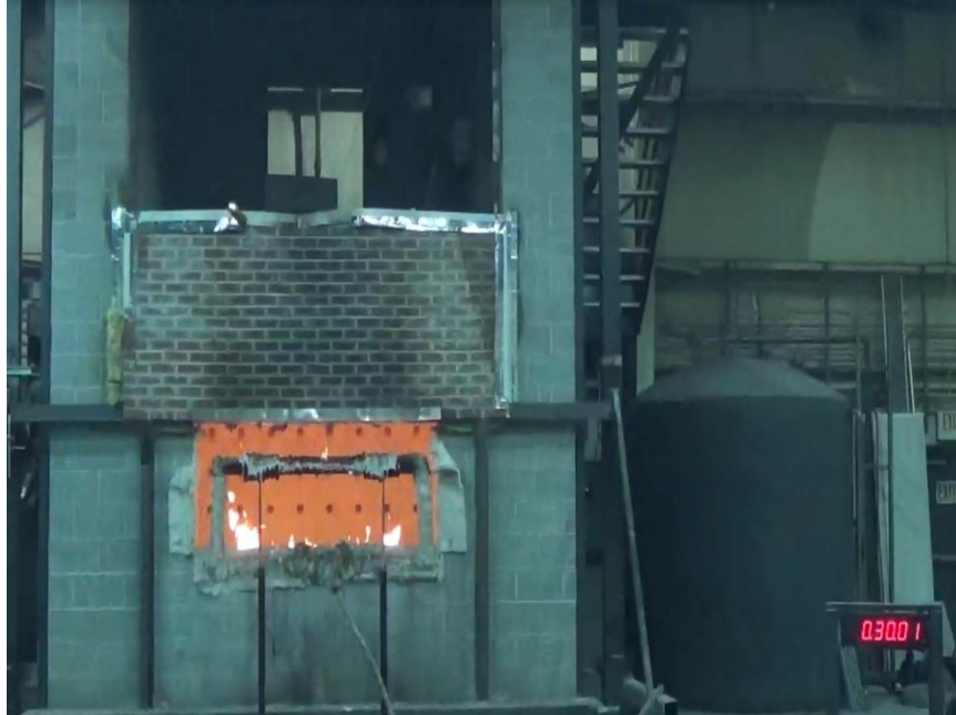
Photo No. 5 Test #2 End of First 30 Minute Exposure
